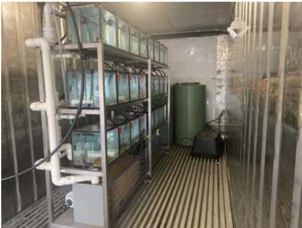
Figure 2. Rack system comprised of 28 x 30L aquaria.
