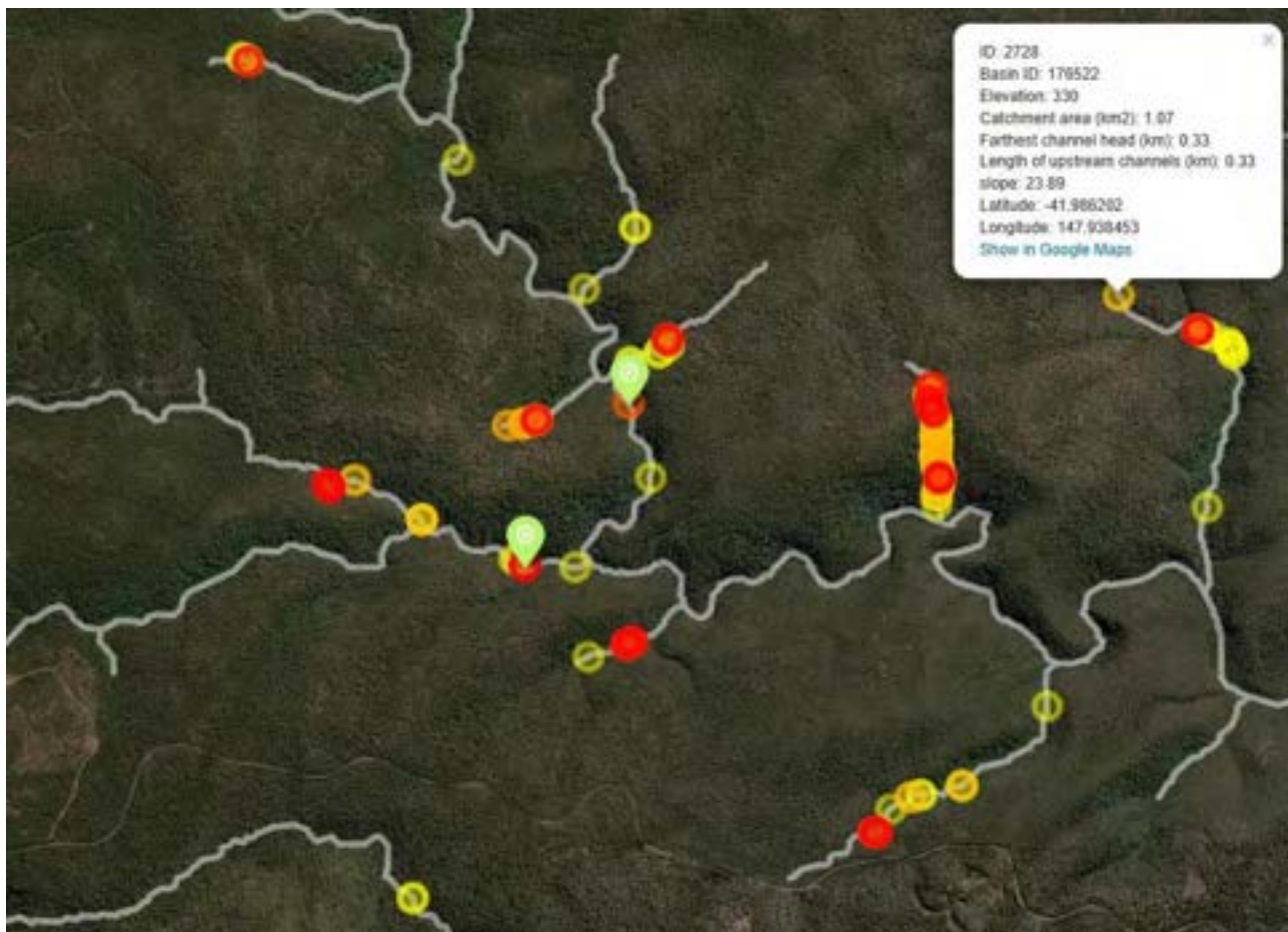
Figure 4. Example output of a DEM-based instream barrier analysis.
