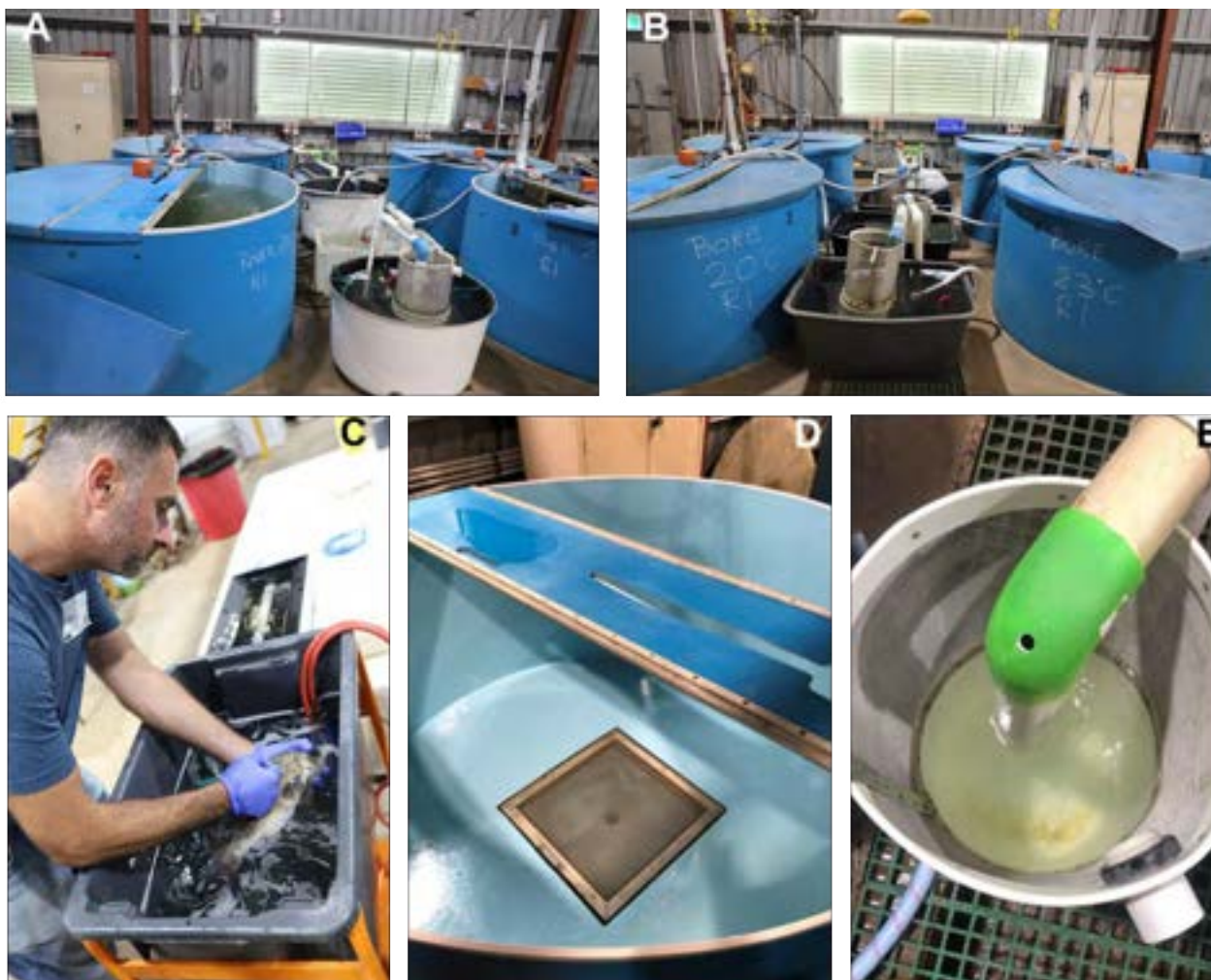
Figure 4. Broodstock spawning tanks and recirculation system for egg collection. River and bore water assigned tanks (A, B); implantation (C); egg collection system (D, E). (Photos by L. Pearce.)
