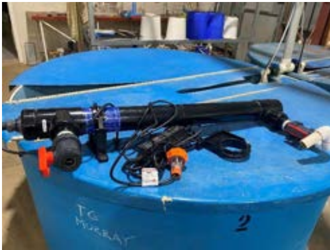
Figure 10. UV Filter that will be installed in recirculating system.
