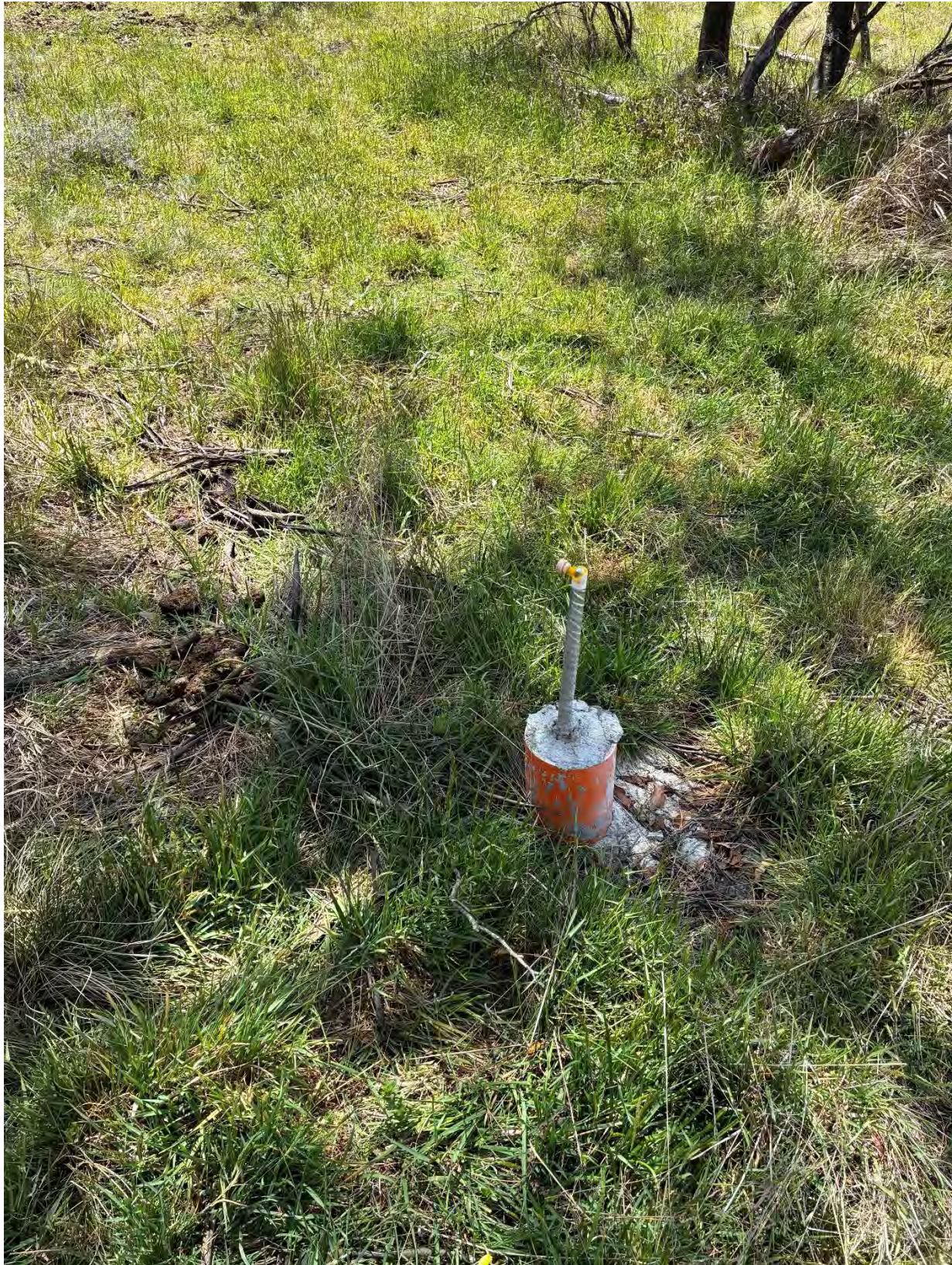
Photograph 12 – Survey monument missing prism
