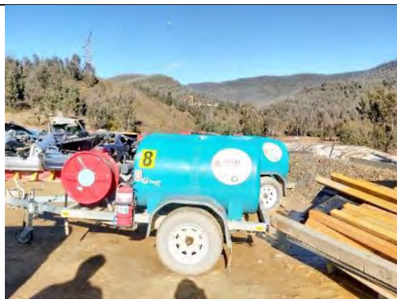
LH 14: Mobile fire fighting water cart at Pad 2. Wrecked vehicles in background are used for practice rescues
