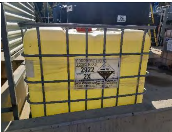
LH 22: Sewage treatment plant UN 2922 (Phenyl isothiocyanate) stored with Sodium hydroxide (base - to right of photo) – incompatible to be stored with acids, bases or oxidising agents.
