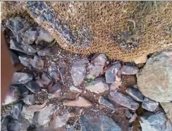
LRR 9: Further close-up of plastic mesh– small pieces breaking off and entering environment
