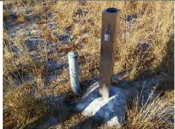
Site 5: Site of 3 water bores including a vibrating wire piezometer (VWP). A weed control program is in place for all bore pads and access tracks – sprayed once to twice yearly using hand spraying techniques and selective weed spray.
