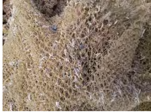
LRR 8: Close-up of plastic mesh – breaking down, releasing plastic pieces into the environment.
