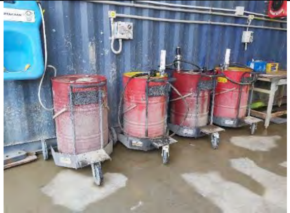
MC31: Workshop area – drums of oil not bunded (refer to overall NC relating to chemicals / bunding management)
