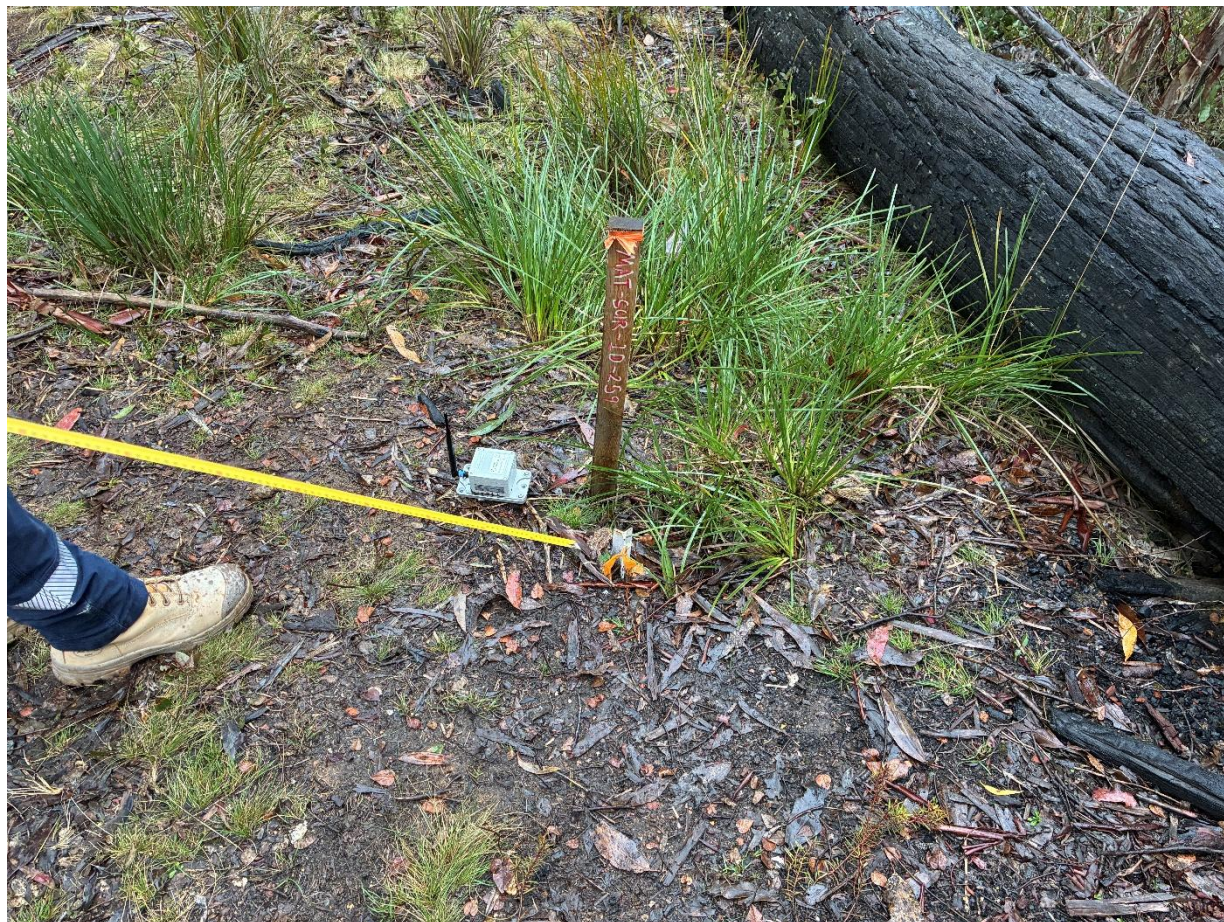
Photograph 4 – monitoring location at CH100 located on the Tunnel centreline. Note Tiltmeter, timber peg with flagging tape, and star picket used for re-levelling
