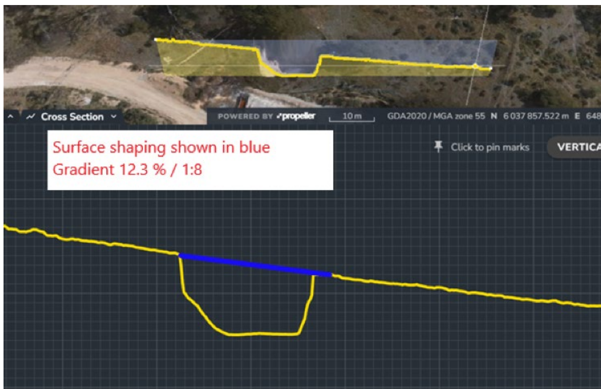
Figure 7: Final landform cross section
