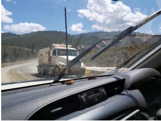
LH15: Water truck – near Main Camp - spraying road for dust suppression
