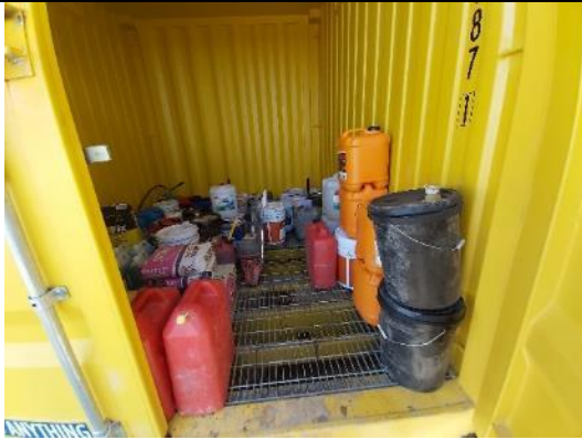
MC13: Inside the flammable storage container – bundled, chemicals / fuels compatible
