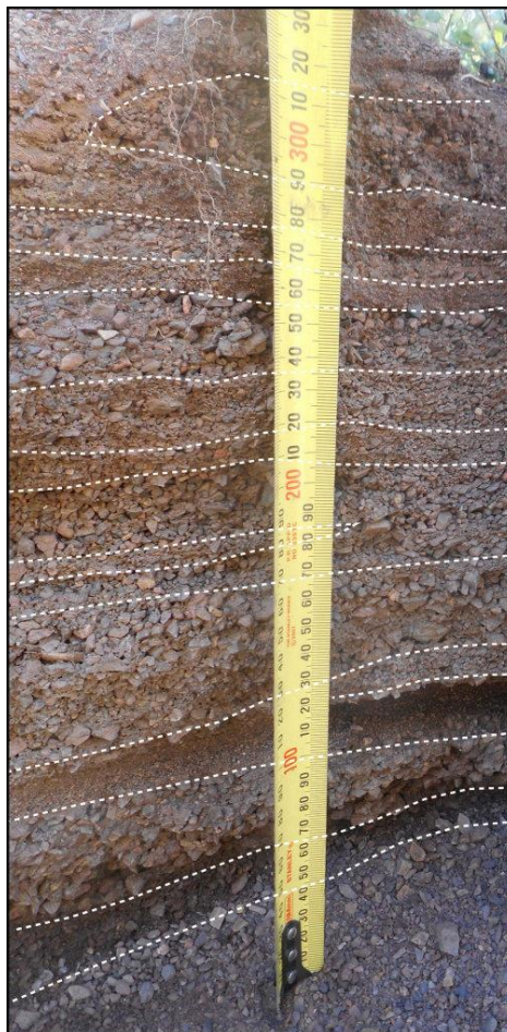
Figure 14 Multi phase proximal overbank sediments near to confluence of Sheep station Creek and small tributary.
