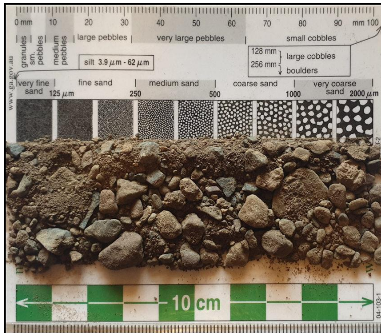
Figure 15. Grainsize of poorly sorted sediment filling detention basin at Lick Hole Gully Site 1
