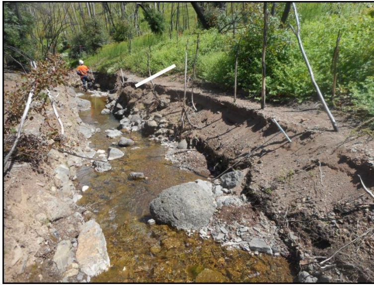
Figure 9 Watercourse 3 shows evidence of recent incision and is scoured to bedrock and has large cobbles and boulders exposed in the base. Proximal overbank deposits shows multiple stages of deposition and incision
