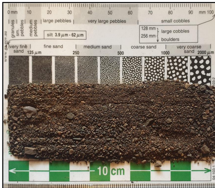
Figure 13 Poorly sorted proximal overbank deposition on small tributary of Sheep Station Creek.
