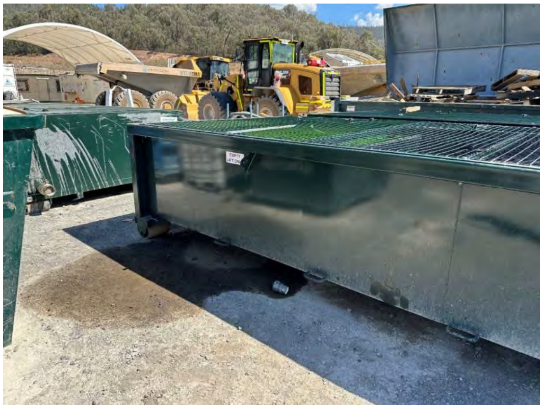
Photo 44 –Spill at coolant waste coolant bin in contractor yard (Main Yard). Note high capacity and not stored as per requirements. See IMP REC 29.
