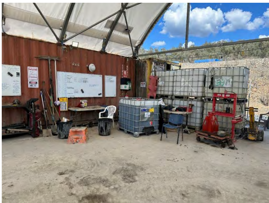
Photo 40 – Contractor yard (Main Yard) hydrocarbons incorrectly stored and not as per AS 1940. See NC REC 14.
