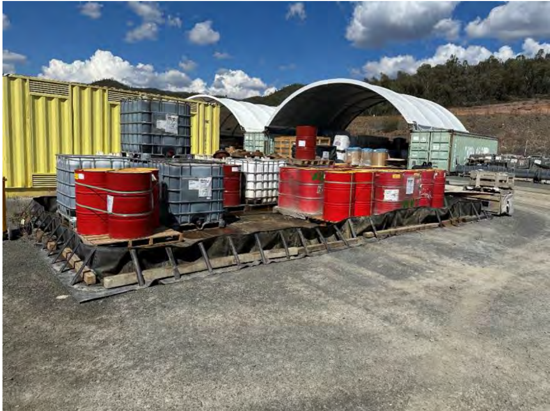
Photo 47 - Contractor yard (Main Yard) hydrocarbons stored in bunding.
