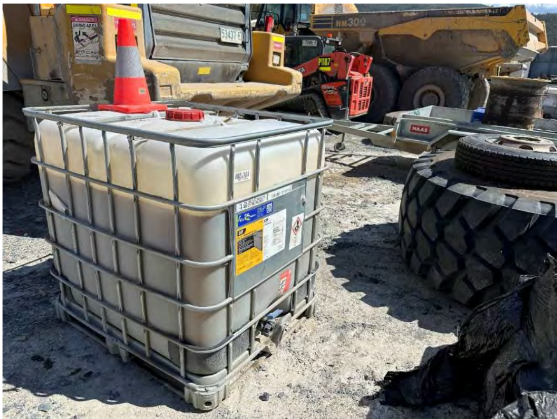
Photo 42 – Contractor yard (Main Yard) hydrocarbons incorrectly stored. See NC REC 14.
