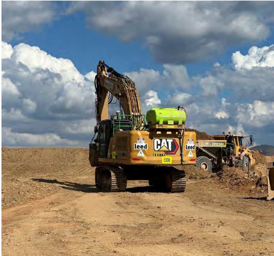
Photo 01 – Plant fitted with water tank and sprayer.
