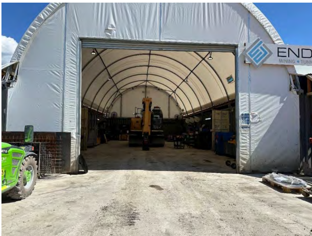
Photo 39 – Contractor yard (Main Yard) workshop without drip trays/bunding. See NC REC 11.
