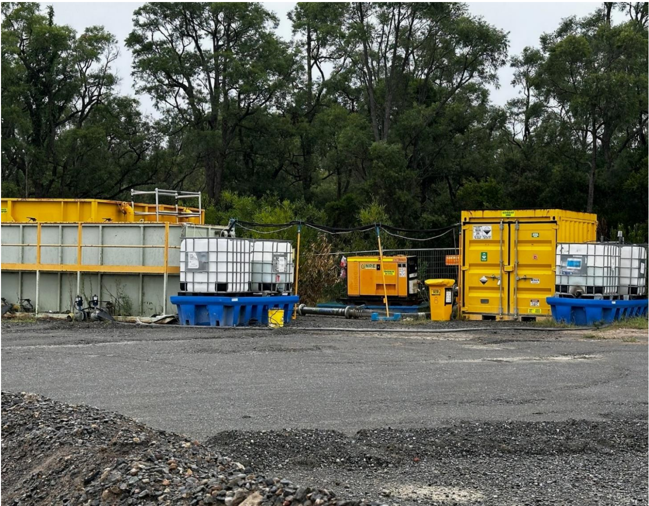
Photograph 12: Bunded and ventilated chemical storage container and mobile bunds
