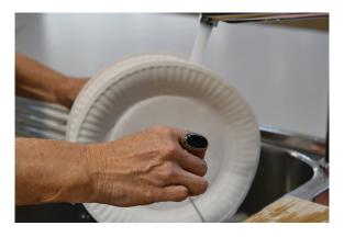
7. Hold your turbine by the ends of the skewer horizontally under the flow of running water (tap) and watch it turn.Alternatively, you can use a bucket instead - see next step
