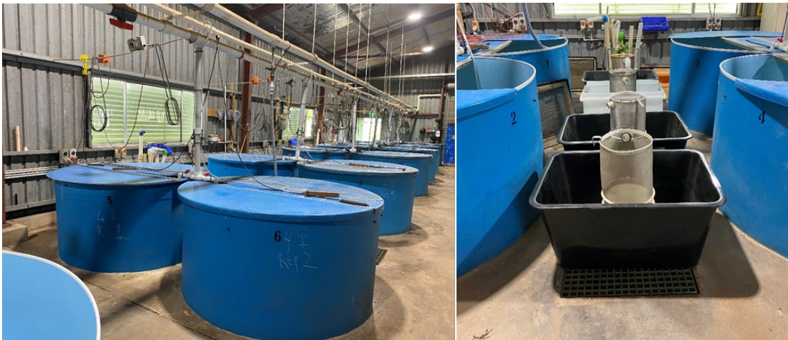
Figure 19. Spawning tanks at NFC with Egg collection sump bank (servicing 4 spawning tanks).
