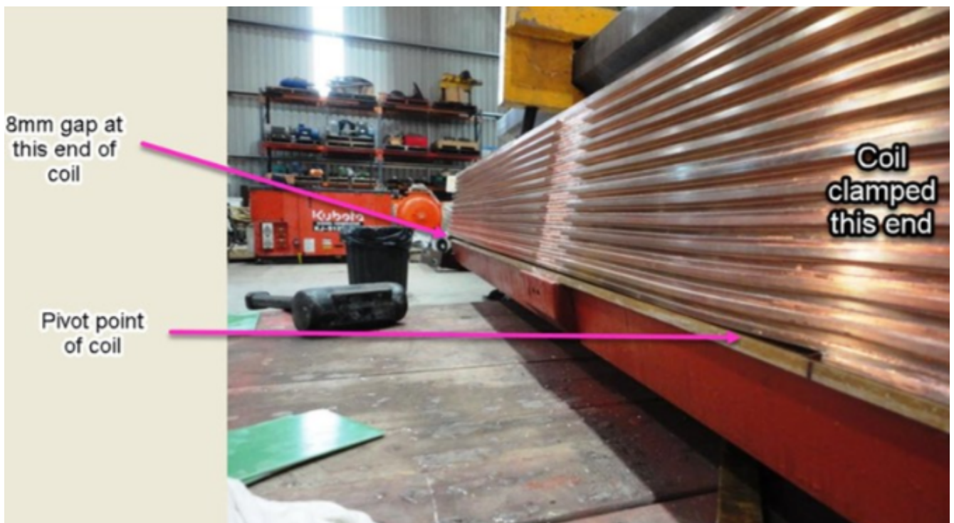
Previous flatness issues on new coils supplied for M1U03 rotor repair in 2018
