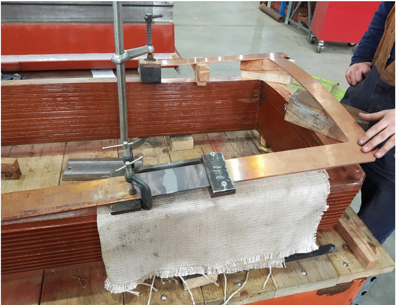
Replaced pole connection showing brazed joints > 400mm from pole connection
