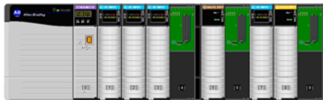
Figure 3.2 - I/O or Secondary Chassis Layout
