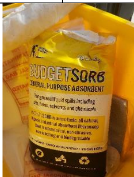
TT17: Organic absorbent is spill kit – STP – may not be suitable for strong corrosives (should be inert absorbent)
