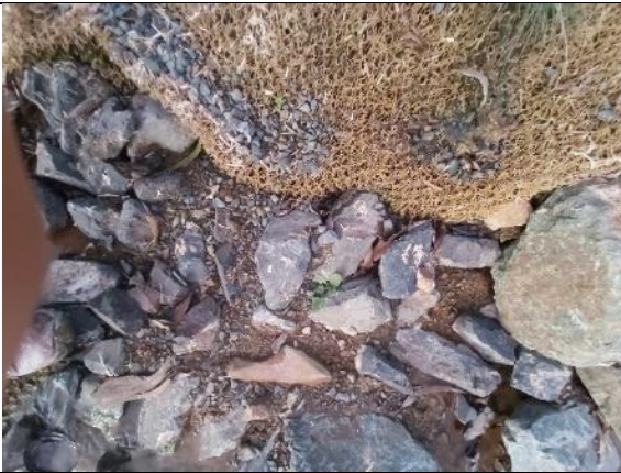
LRR 9: Further close-up of plastic mesh– small pieces breaking off and entering environment
