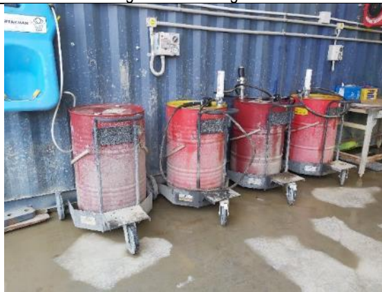
MC31: Workshop area – drums of oil not bunded (refer to overall NC relating to chemicals / bunding management)
