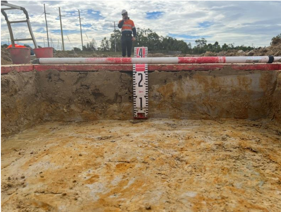
Plate 6 Square 1, NNE section. Note light brown sandy intrusion to a depth of c. 18 cm.
