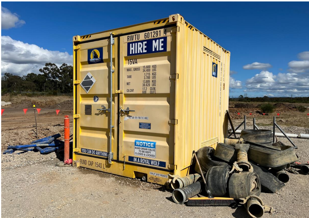
Photograph 8 - Self Bunded Fuel and Chemical Storage Container
