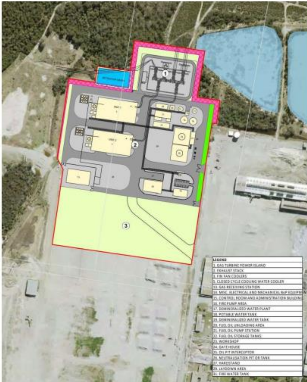
Figure 1-2: Approved Project EIS boundary (red line) and overlay of Power Station Infrastructure
