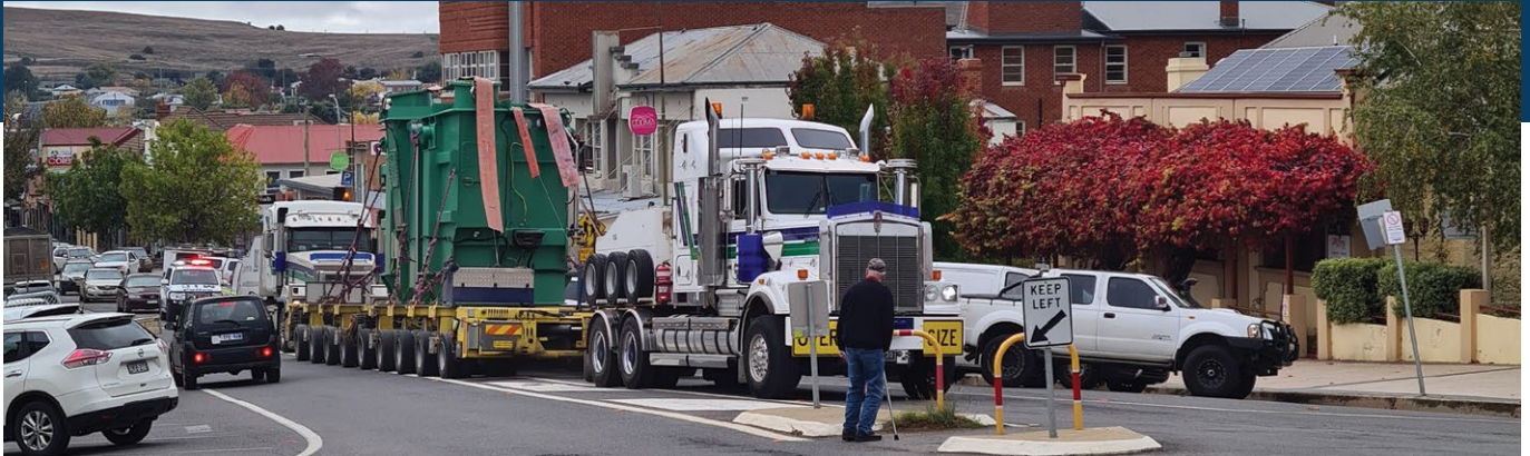
A transformer on its way to Cabramurra for the new substation
