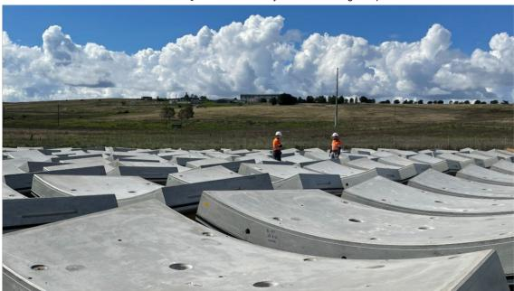
Production is well underway at the precast factory at Polo Flat, Cooma, with hundreds of huge concrete segments lined up in the storage yard ready to be transported. Viewed from above, the precast segment factory is a telling example of the scale and complexity of the Snowy 2.0 project.
