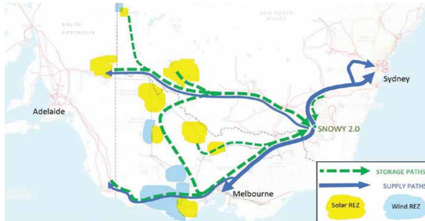
Illustration showing existing and proposed solar/wind energy development and how they would relate to Snowy 2.0. This also shows how Snowy 2.0 connects to the main load centres north and south.
