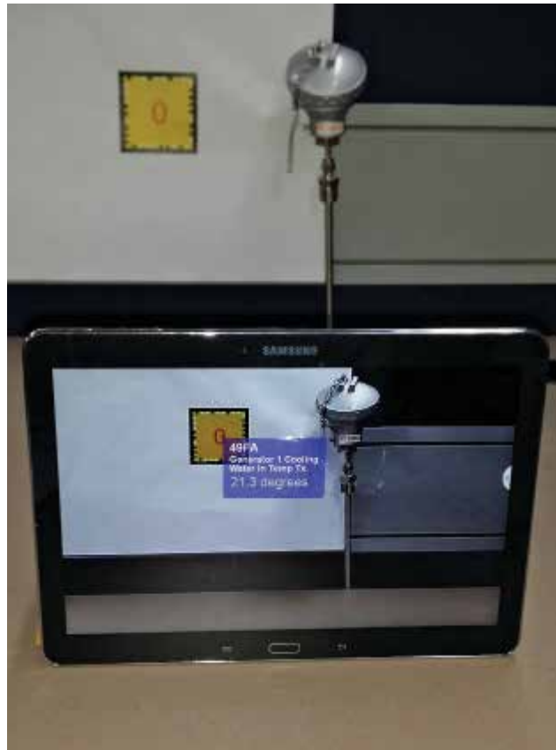
Augmented reality is supplementing what you can actually see with an overlay of virtual information. Using a camera in the smart device pointing at an augmented reality marker (the square), real time data can be displayed using a specialised app. The real time data is streaming from automation systems associated with the asset.
