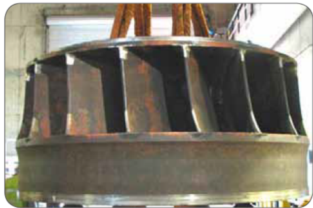
The old runner being removed from Tumut 3, one can be seen in the exterior display at the Snowy Hydro Discovery Centre in Cooma.
