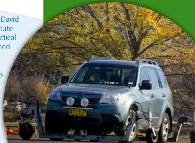
The skid car in action.
